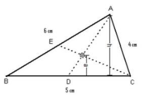
The center of gravity is at the intersection of lines BE and AD. The distance a can be calculated as
