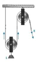
(ii) The purpose of the pulley Q is to change the direction of application of effort to a convenient direction.
